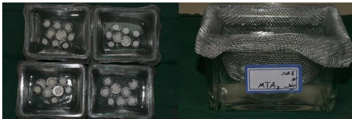
Figure 1: The containers with experimental ring moulds immersed in STF. Each mould has a code to record its weight before and after the immersion time period.
