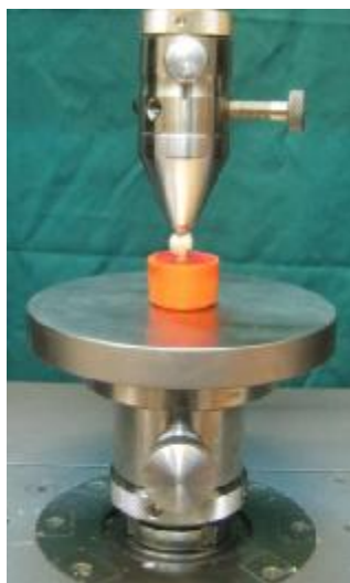
Figure 4: Frontal view of specimen positioned in the universal testing machine
