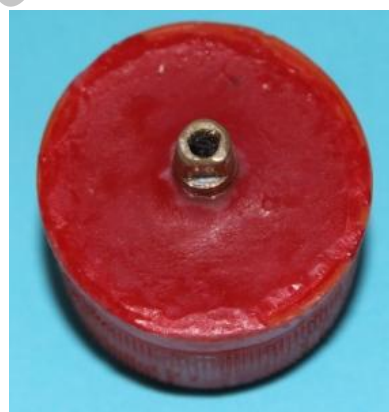
Figure 1: Brass die embedded in acrylic resin block
