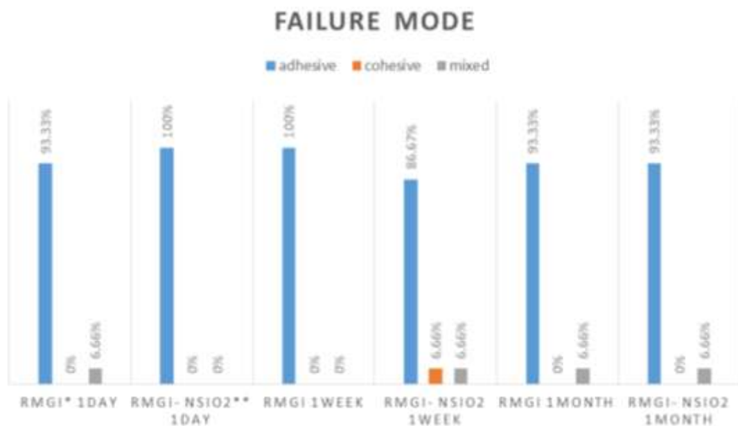
Figure 1: Frequency bar chart of fracture modes of two sample groups at three different intervals
