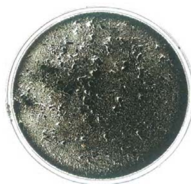
Fig. 11a. Granules obtained from HUASB reactor
