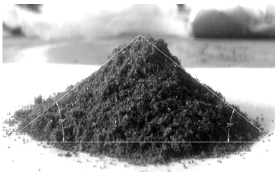
Fig. 1. Tracing lines on diagonal faces of compost triangle
