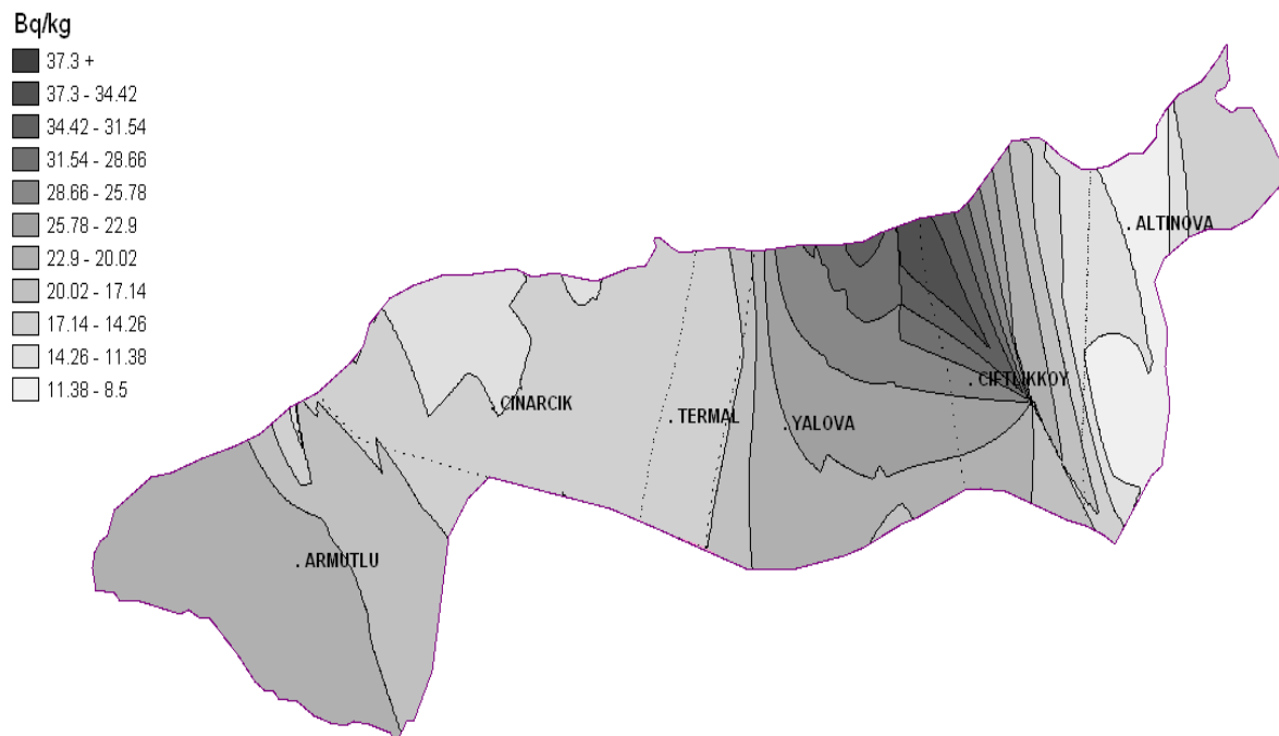
Fig. 4. The map of ^{238}\text{U} radionuclide activity concentrations
