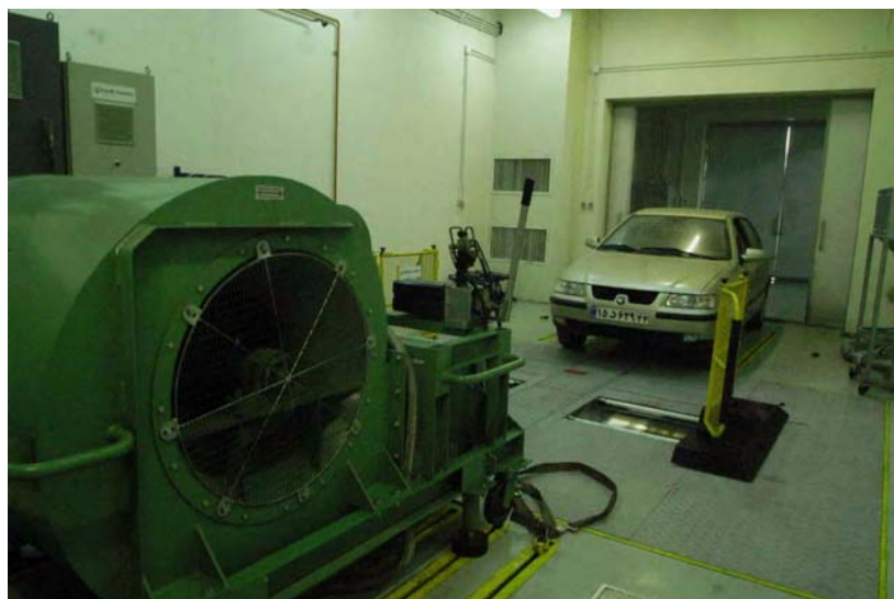
Fig. 6. Experimental setup containing a dynamometer chassis and an exhaust emissions analyzer
