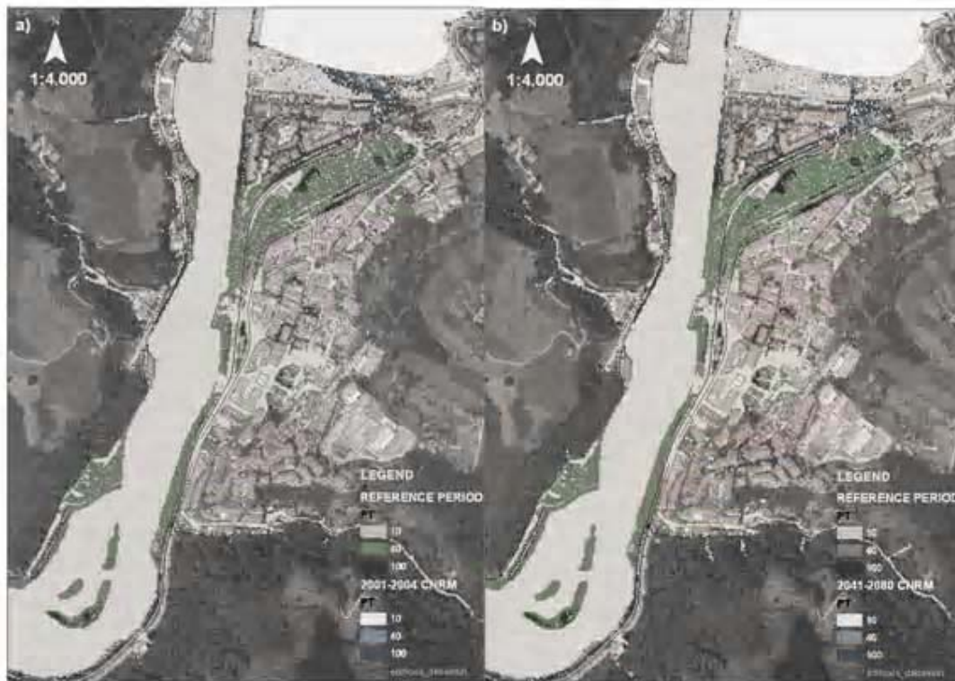
Fig. 4. a) Flood extent map. Actual (reference period, 1961-200) and future (with CC, 2001-2040). CNRM model. b) Flood extent map. Actual (reference period, 1961-2000) and future (with CC, 2041-2080). CNRM model
