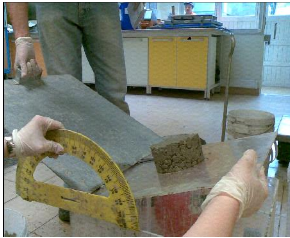
Fig. 4. Inclined plane test
