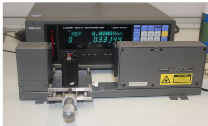
Figure 1. Travel crossed roller table connected to a micrometre perpendicular to the scanning laser beam of a laser scan micrometer. D_0 level was established as a first reading achieved by LSM, where the specimens touched the laser beam; consequently, specimens were moved manually using micrometre ruler for further measurements
