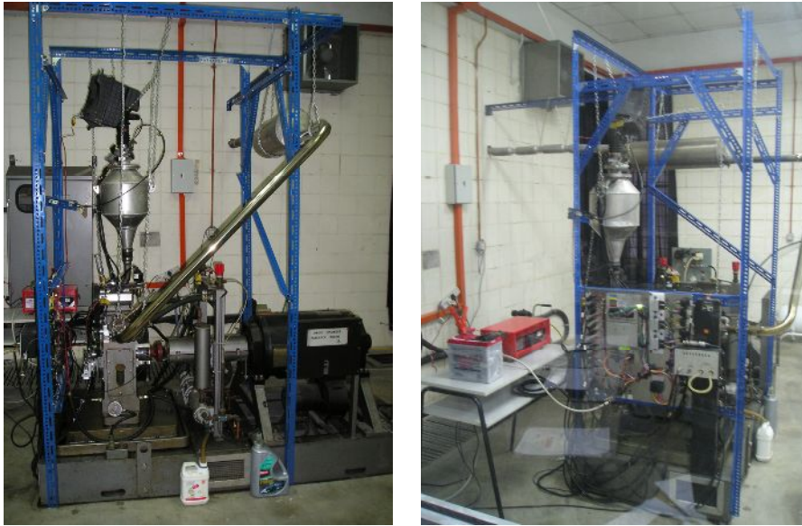
Fig. 29. The SCRE test rig of CNG-DI engine.
