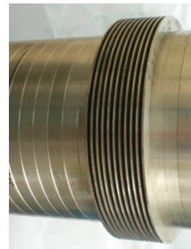
Fig. 3. Internal part (insert) with 11 teeth.
