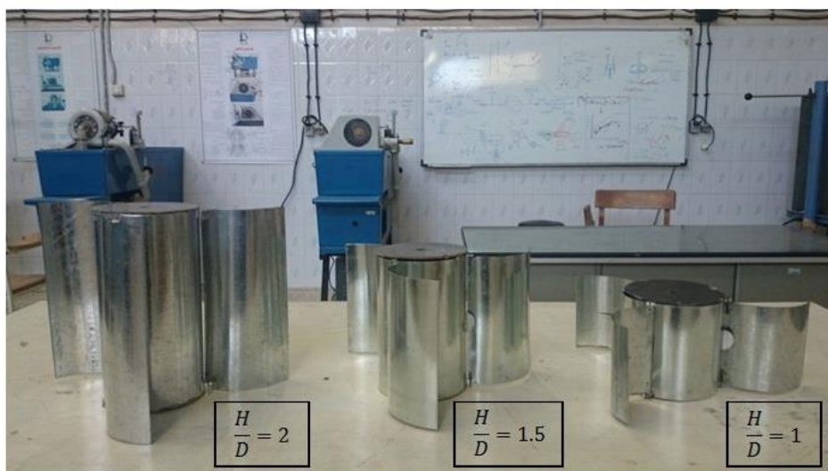
Fig. 4. 3-bladed rotors with various aspect ratios used in the experimental measurements.
