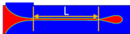
Fig. 17. Location and dimension of the droplet breakup point. The heating temperature of the dispersed phase is 10°C, the inlet temperature of the left and right oil phases is 20 and 30 °C, respectively.
