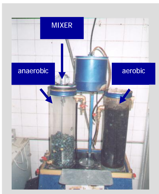
Figure 1- The two anaerobic- aerobic reactors
