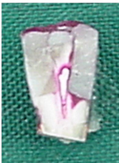
Figure 3. Dye penetration under the layer of fluid composite. Score 0 = no dye penetration (right), score 4 = dye penetration past the axial wall (left).
