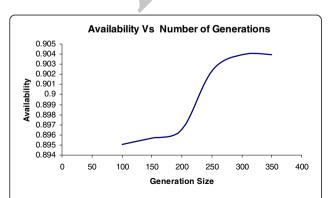
Figure 3 Effect of number of generations on crystallization unit availability.
