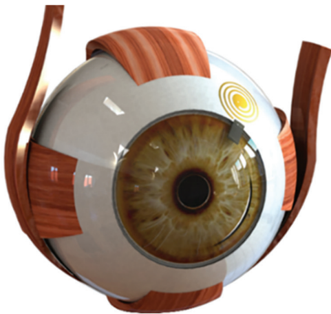
Figure 2. A three-dimensional model of the eye showing an implantable capacitive IOP sensor integrated into the anterior chamber; the antenna of the sensor is placed in the sclera. IOP, intraocular pressure
