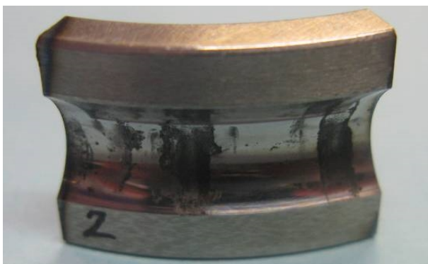
Figure 11: False brinelling in the inner race of an angular contact ball bearing
