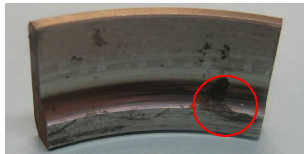
Figure 4: Fatigue damage on an angular contact ball bearing outer race
