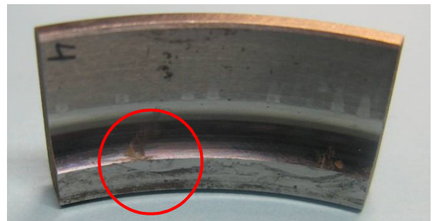
Figure 8: Abrasive wear in an angular contact ball bearing
