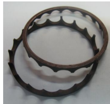
Figure 17: Failure of an angular contact ball bearing cage
