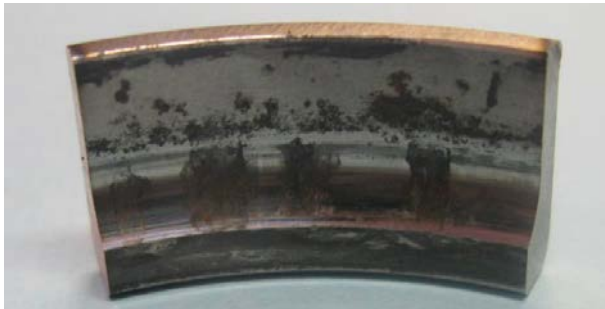
Figure 10: False brinelling in the outer race of an angular contact ball bearing
