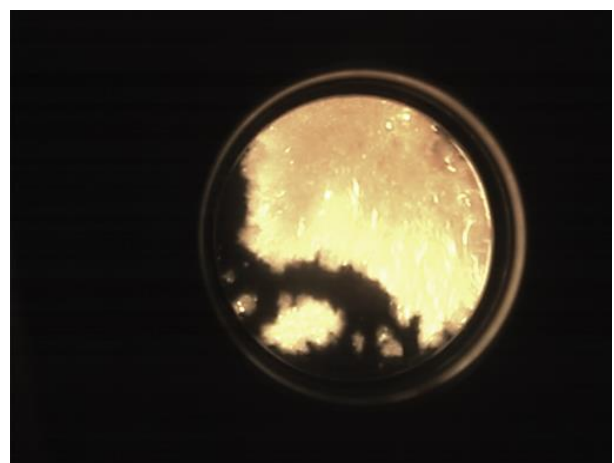
Figure 12: Blown-up intensified view of the multiple auto-ignition initiation sites observed during the baseline heavy knock cycle
