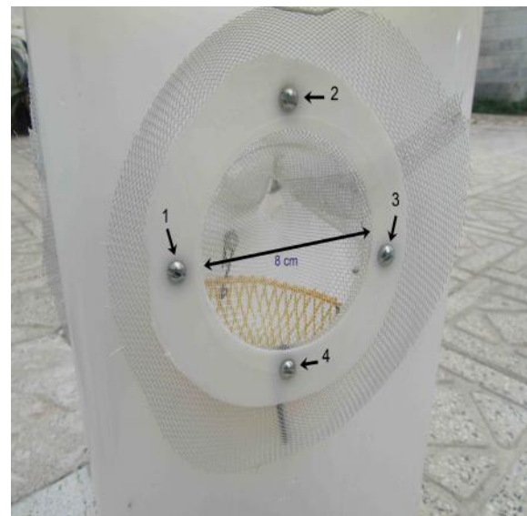
Fig. 3. Round openings of the modified adult flytrap with 8cm in diameter, provided for one-way entering flies, Tehran University of Medical Sciences, 2010 (original)
