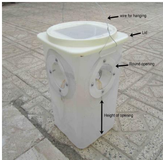
Fig. 2. A Modified adult fly trap, evaluated as an applicable trap for collecting various families of Diptera, Fars Province, Iran 2010 (original)
