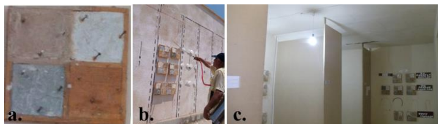
Fig. 1. a. Wooden container with four different surfaces, b. Spraying operation, c. Install contain after spraying in room which separated into four parts
