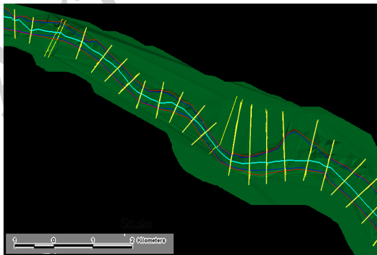
Fig6. Flow path, bank and cross section cut line themes prepared using the preRAS option
