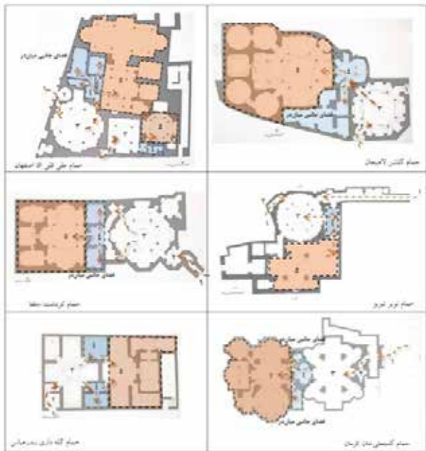
Fig. 6. The presentation of the three spaced structure derived from 9 Iranian historical public bathes. Source: Haji Ghasemi, 2004.
