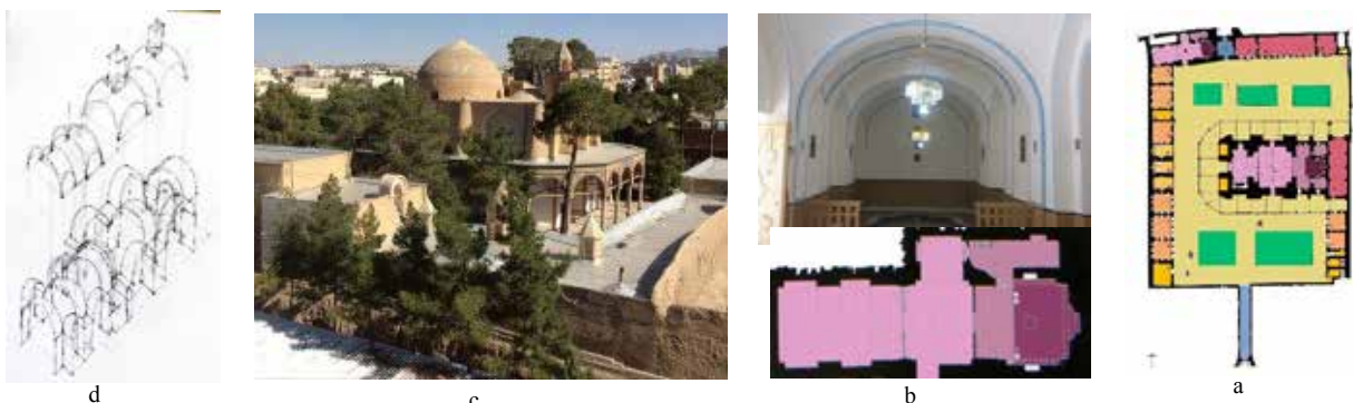
Fig. 6. The location, plan, and the vaults composition of St. James Church. Source: authors archive; Haghnazarian, 2006.
