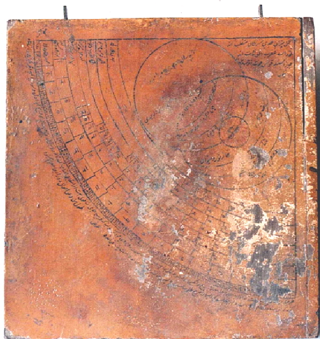
Fig. 7: Shabnumā-wa-Rūznumā , Reverse showing a Horary Quadrant as the Rūznumā . Raza Library, Rampur.
