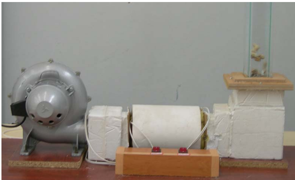
Fig.1. Lab scale fluidized bed dryer
