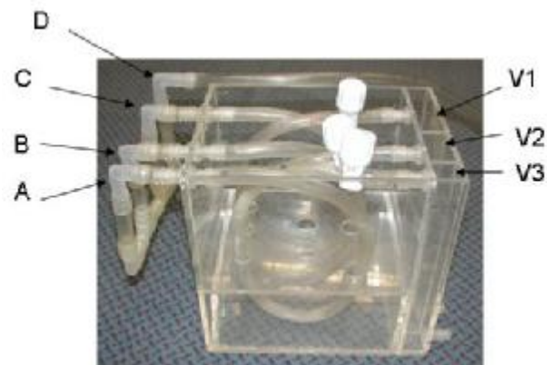
Fig 5- Picture of MR flow phantom. The phantom contains three branches. A, B, C and D contain four different flow rates. V1, V2 and V3 are the effective volumes for measuring different flow rates.
