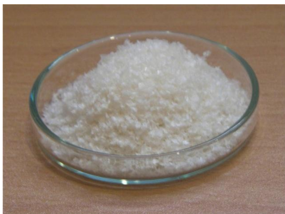
Figure 3. Prepared chitosan from shrimp shells in Nanomedicine and Tissue Engineering Research Center
