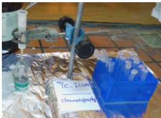
Figure 3. Chromatography set-up (Sephadex) for labeled ICD-85 separation
