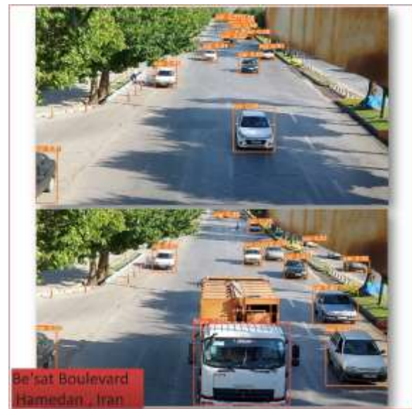
Figure 16. The result images from the processing of the traffic control camera installed in Be'sat Boulevard, Hamadan, Iran by the algorithm developed in this article.
