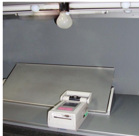
Figure 1: The experiment setup for measurement of lighting source characteristics.
