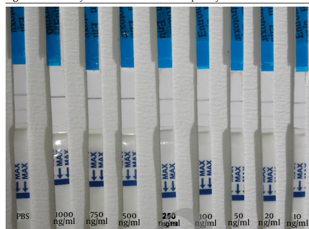
Figure 1. Sensitivity of the Sandwich-Based Strip Assay for the Detection of SEB
