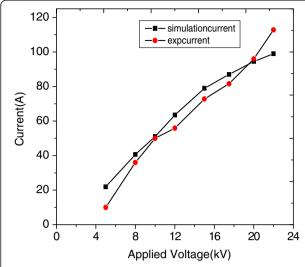
Figure 7 Beam current (simulation and experimental) for different applied voltages at z = 0 mm.
