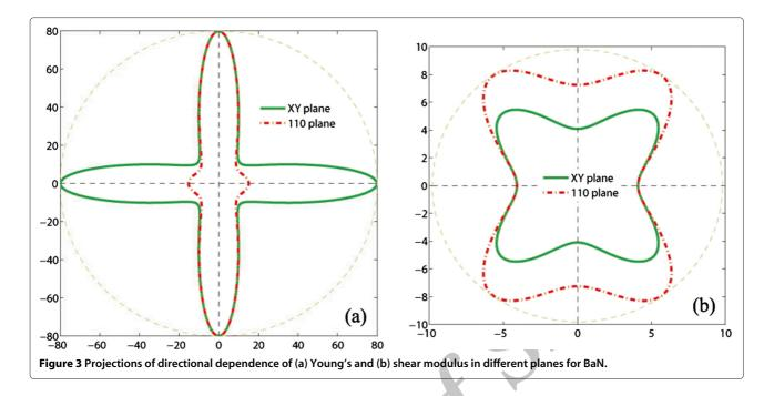
elastic anisotropy theoretically. For example, the so called Zener's anisotropy parameter  $A=2C_{44}/(C_{11}-C_{12})$  is widely used for this purpose [15,16]. The degree of deviation of Zener's anisotropy parameter from unity 1 indicates the degree of elastic anisotropy. SrN is nearly elastically isotropic with A=0.79, and a higher degree of elastic anisotropy is found in BaN with A=0.13, as listed in Table 3.
