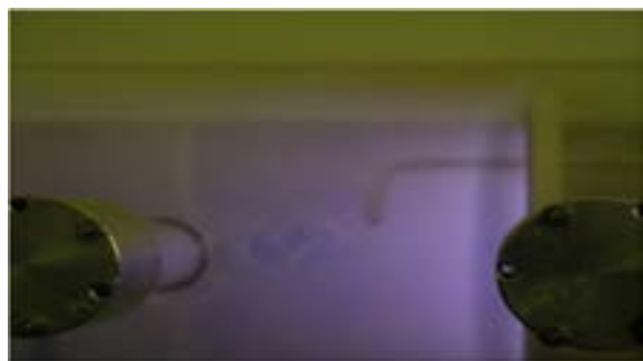
Figure 3 Plasma and Langmuir probe in the discharge tube close to the cathode.
