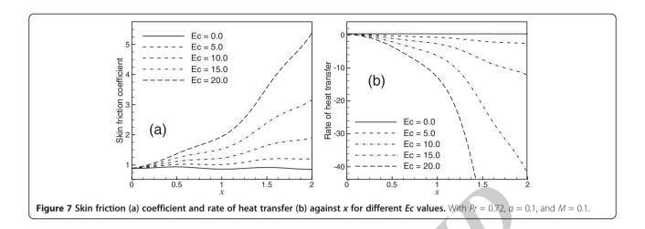
Figure 7b that for higher values of the Eckert number *Ec*, the rate of heat transfer decreases, that is, heat transfer slows down significantly for higher Eckert number *Ec*.
