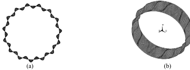
Fig. 1 FE first eigen buckling mode shape in (a): front view and (b): isometric view.
