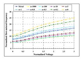
Fig. 5 Effect of normalized voltage to first natural frequency for various FGM indexes ( $T^{*=0}$ )
