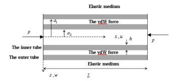
**Fig. 1** A double-walled carbon nanotube embedded in an elastic medium.
