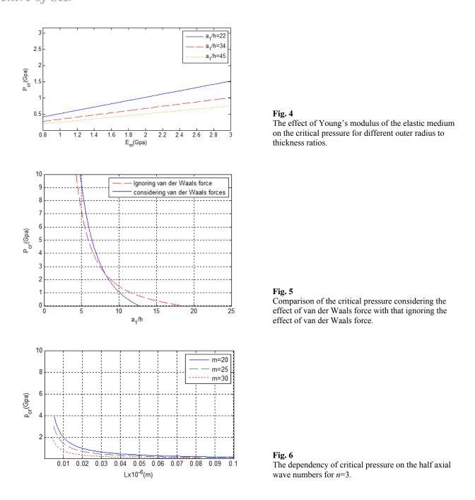
Fig. 6 shows the variation of the critical buckling load  $p_{cr}$  with respect to the tube length (*L*) for various axial half wave numbers 20, 25 and 30 (*n*=3). As can be seen from this figure that the critical buckling load decreases with increasing of the length of the nanotube for a constant radius of the outer tube ( $a_1$ ). It is also observed that the critical pressure descend very quickly with increasing the half axial wave numbers.
