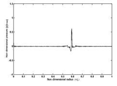
Fig. 6 Non-dimensional pressure distribution due to input  $p(1,t) = 10^{-3} p_o \delta(t)$  at non-dimensional time  $\hat{t} = 0.4$ .
