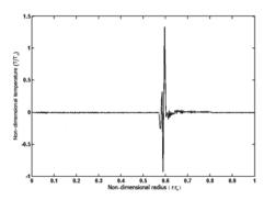
Fig. 5 Non-dimensional temperature distribution due to input  $T(1,t) = 10^{-3}T_o\delta(t)$  at non-dimensional time  $\hat{t} = 0.4$ .
