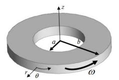
Fig. 1 Geometry and boundary conditions of an FGM piezoelectric disk.
