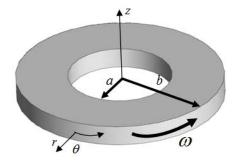
Configuration of thin-walled finitely radius of the EGM hollow rotating disk.
