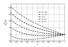
**Fig. 8** The radial stress distribution along the radius in the EGM hollow rotating disk (fixed-free boundary conditions) for different values of *K*.
