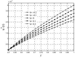
**Fig. 7** The radial displacement distribution along the radius in the EGM hollow rotating disk (fixed-free boundary conditions) for different values of *K*.
