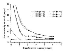
Phase velocity profiles of wave modes in a stress free thermally insulated plate with circumferential wave number.
