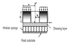
Fig. 1 Geometry of FGMs annular plate with clamped-clamped supports resting on two parameter elastic foundations.
