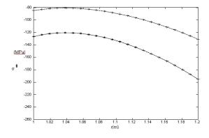
Fig.27 Radial thermal stress in the cross section of cylindrical.
