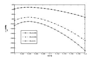
Fig. 31 Shear thermal stress in the cross section of cylindrical.
