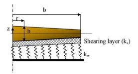
**Fig. 1** Geometry and foundation parameters of the two-directional functionally graded variable thickness circular plate.
