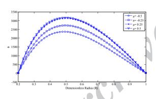
Fig. 9 Distribution of the electric potential versus the dimensionless radius of the disk for fixed-free boundary conditions,  $T_{in} = 0$ °C and  $T_{out} = 30$ °C.
