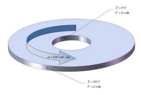
**Fig. 1** Configuration of a radially polarized FGPM rotating disk.
