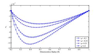
Distribution of the dimensionless radial stress versus the dimensionless radius of the disk for free-free boundary conditions,  $T_{in} = 0$ °C and  $T_{out} = 30$ °C.
