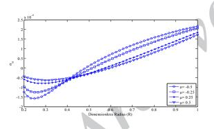
Fig. 5 Distribution of the dimensionless circumferential stress versus the dimensionless radius of the disk for fixed-free boundary conditions,  $T_{in} = 0$ °C and  $T_{out} = 30$ °C.
