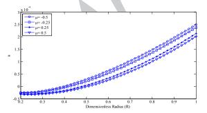
Fig. 10 Dimensionless radial displacement versus the dimensionless radius of the disk for free-free boundary conditions,  $T_{in} = 0$ °C and  $T_{out} = 30$ °C.
