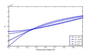
Fig. 4 Distribution of the dimensionless circumferential stress versus the dimensionless radius of the disk for free-free boundary conditions,  $T_{in} = 0$ °C and  $T_{out} = 30$ °C.
