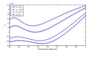
**Fig. 7** Distribution of the dimensionless von Mises stress versus the dimensionless radius of the disk for fixed-free boundary conditions,  $T_{in} = 0$ °C and  $T_{out} = 30$ °C.
