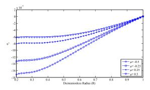
Fig. 3 Distribution of the dimensionless radial stress versus the dimensionless radius of the disk for fixed-free boundary conditions,  $T_{in} = 0^{\circ}\text{C}$  and  $T_{out} = 30^{\circ}\text{C}$ .
