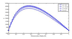
Fig. 8 Distribution of the electric potential versus the dimensionless radius of the disk for free-free boundary conditions,  $T_{in} = 0$ °C and  $T_{out} = 30$ °C.
