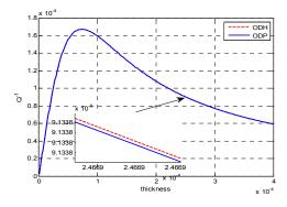
**Fig. 3** Comparison of  $Q^{-1}$  for Parabolic and Hyperbolic heat conduction model for R/h=50 and  $T_{\circ}=300$ .
