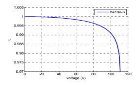
Fig. 6 Effect of DC voltage on  $\xi$  for  $h = 10 \ \mu m$  and  $E = 250 \ \mu m$ .
