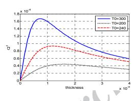
**Fig. 4** Effect of the plate thickness on  $Q^{-1}$  for different ambient temperatures (R/h=50).
