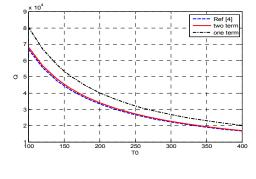
**Fig. 2** Comparison of Q for different temperatures,  $h = 10 \ \mu m$  and R/h=50.
