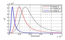
**Fig. 5** Effect of plate radius on  $Q^{-1}$  for different thicknesses.
