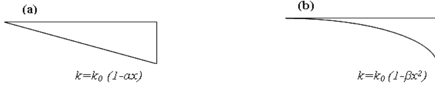
Fig. 2 Various Winkler elastic foundations along the axial direction: (a) linear type (b) parabolic type.
